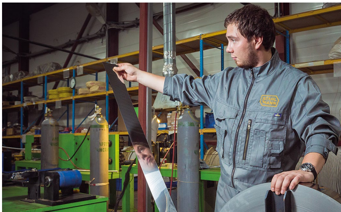
SS304 stainless steel tape used in the manufacture of corrugated tubes
