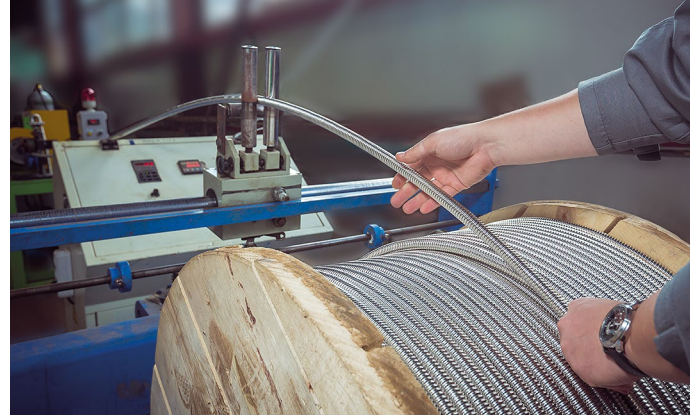
Stahlmann corrugated tube fed for annealing
